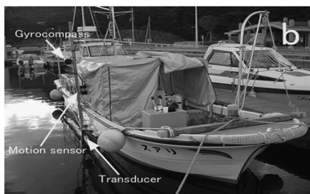
Fig. 1. Schematic view of multi-beam sonar (a) and photograph of R/V Rias equipped with the multi-beam sonar, gyrocompass and motion sensor utilized for mapping seagrass beds (b). Map of Otsuchi Bay on the Sanriku Coast facing the Northwestern Pacific (left panel) and the study site off Nebama in Otsuchi bay (right panel).
