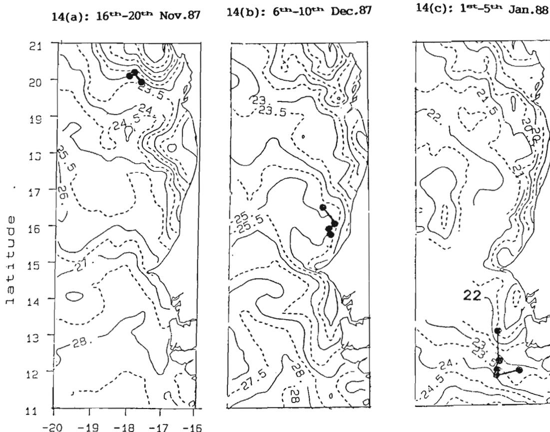
**Figure 15.** – Exact locations of the daily catches (by 5 days periods) and corresponding sea surface temperature measured by Meteosat satellite (processing made by the UTIS laboratory, courtesy of Mrs Marec and H. Demarcq) for a school exploited between November 1987 and January 1988. 15 (a): 16<sup>th</sup> to 20<sup>th</sup> of November 1987. 15 (b): 6<sup>th</sup> to 10<sup>th</sup> of December 1987. 15 (c): 1<sup>st</sup> to 5<sup>th</sup> of January 1988.
