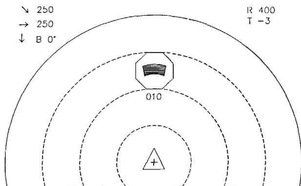
**Figure 2.** – Estimate function of the Furuno CSH-70 (R: search range of sonar, T: tilt angle, arrows: slant, horizontal and vertical distance to marker, B: direction of bearing to marker).
