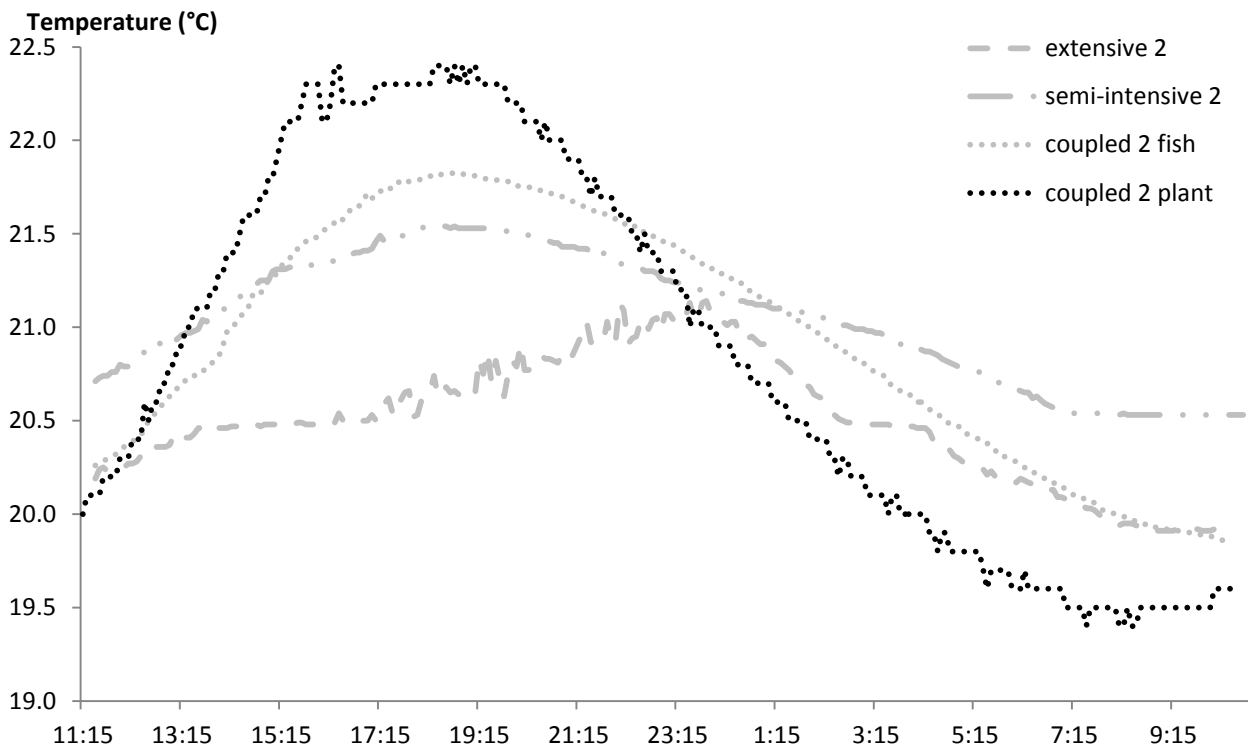
Figure IV. Water temperature measured at a depth of 50 cm every 5 minutes for 24 hours in September 2014 in pond 2 of each treatment
